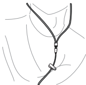
1. Shirt clip holds cable in place
